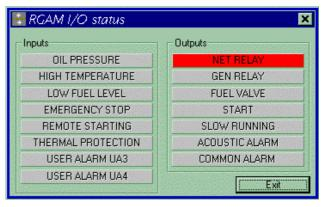
When one of these boxes is highlighted in red, it means that the corresponding I/O is active. It is important to understand that the red color does not indicate the status of the contact but the 'active' state, that is the contrary of the one at rest. For instance, the emergency stop input, which is connected to a normally closed contact, will be highlighted in red when the contact opens (condition that generates the emergency condition)
